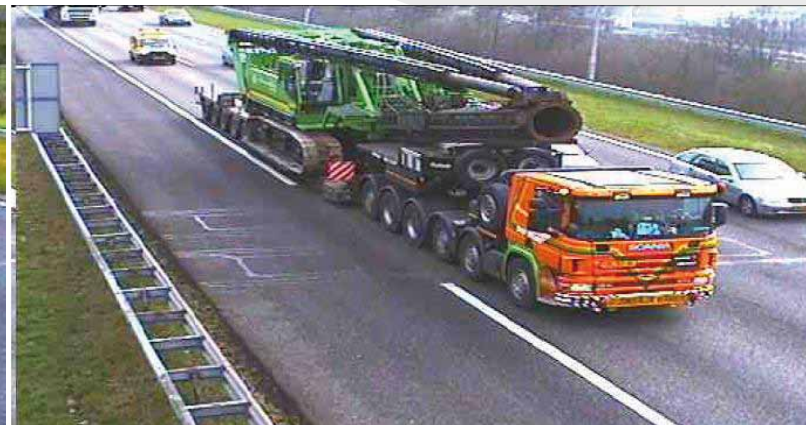
Figure 2.2 Low-loader vehicle with a total weight of 1450 kN
