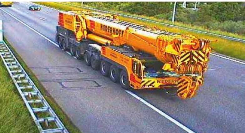
Figure 2.1 Axle crane with a total weight of 1110 kN
